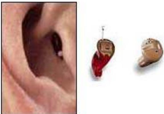
Even smaller is the **completely-in-the-canal hearing aid**, which is virtually invisible when worn. Again, because of its small size, its casing is too small to be able to hold a very powerful amplifier and so it is only useful for mild hearing losses.
