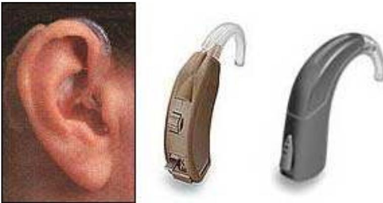
The most commonly used type of aid is the **behind-the-ear hearing aid**, where all the electronic components are contained in a skin-coloured plastic case that sits behind the ear.
